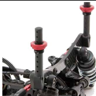
These Aluminum body height adjuster realize fine tunes of height adjustment accurately for bodyshell.
