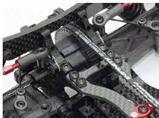
Adjust the chassis flex by connecting this carbon brace between the upper bulkheads on top of the top deck.
